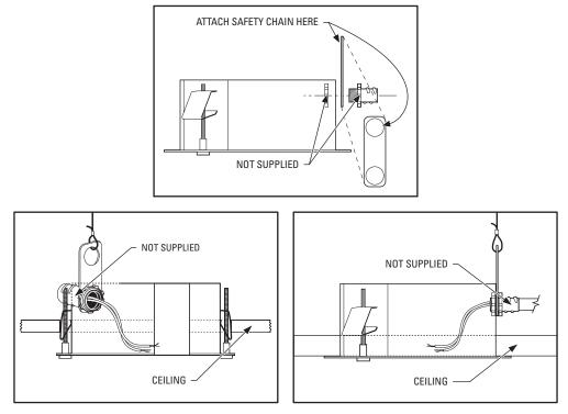
Figure 2. Installing the Back Box
